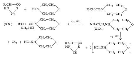
Whereas in presence of aqueous acids these revert to the original thiazolones, under anhydrous conditions carbon disulphide is liberated and the corresponding amides (XX) are obtained. By use of  $\alpha$ -amino-esters this behaviour has, with modifications, been developed into a new method for the controlled synthesis of polypeptides. This may best be illustrated by reference to an example.
