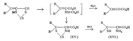
When the thiothiazolidones were heated with hydrochloric acid they were converted into substituted cysteines (XVI), many of which have so been synthesised. Cysteine itself was obtained by a modified procedure whereby 2-mercaptothiazolone was condensed with ethyl orthoformate to give an ethoxymethylene derivative (XVII), which was reduced and rearranged to the desired thiothiazolidone (XVIII) by sodium amalgam (Chatterjee, Cook, Heilbron, and Levy, Part VII, J., 1948, 1337).
